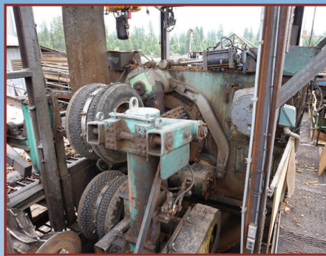
CAMBIO MODEL 30 30' 6-ARM RING DEBARKER
